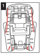
From bottom of shell, release the elastic straps at the bottom of seat and the large elastic straps on the side of seat.
